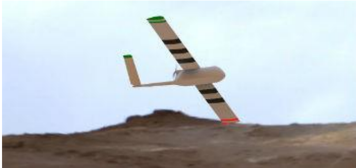
M-10: This available drone model can fly missions up to 14 hours in length.
