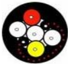
Liquid Hydrocarbon Detector Cables. Geo-location of Leak
