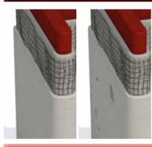
Certification rules dictate that mesh reinforcement has to be installed at a specific depth within the PFP coating, typically at the middle. If the mesh is not installed at the correct depth, the applied system will not meet the requirements of the product's fire certification.
