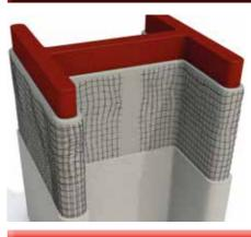
The mesh reinforcement has to be installed in accordance with strict certification rules depending on fire scenario. Following system installation it is very difficult to observe if the mesh has been installed in compliance or installed at all. Incorrect overlaps or lack of mesh will result in unpredictable fire performance.
