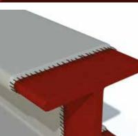
If system terminations are not completed correctly, mesh strands can protrude from the termination point. These exposed strands provide a path for moisture into the coating, leading to poor adhesion, water uptake and reduced fire performance through the life of the system.
