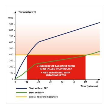
Jotun introduces Jotachar JF750, the industry's first mesh free next generation solution for hydrocarbon and jet fires. Jotachar JF750 incorporates an advanced fibre matrix, eliminating the need for complex mesh reinforcement. When exposed to a fire, Jotachar JF750 produces a robust and temperature stable insulating char whilst risks associated with incorrect mesh installation are eliminated.
