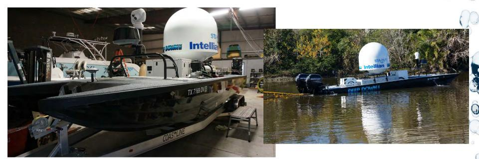
RSV loaded with gyro stabilizer, genset, thrusters,300hp of Mercruisers, thermal cameras, Intellian world wide satellite, remote via link from anywhere. Plus transmit live video feed
