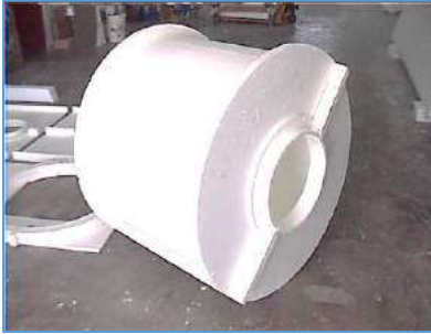
A foam cut-out for trial fitting to a flange
