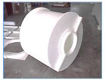
A foam cut-out for trial fitting to a flange
